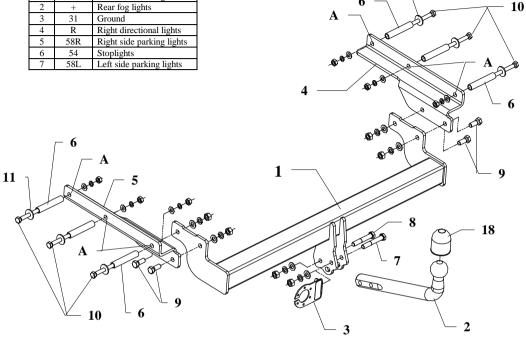
towbar is designed to assembly in following This cars: FORD MONDEO ESTATE, produced since 1993 till 07.1996, catalogue no. C14 and is prepared to tow trailers max total weight 1800 kg and max vertical load 75 kg.
