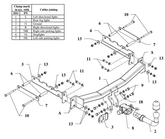
This towbar is designed to assembly in following cars: FORD MONDEO, 4-5 doors, produced since 09.1996 till 09.2000, catalogue no. C19A and is prepared to tow trailers max total weight 1800 kg and max vertical load 75 kg.
