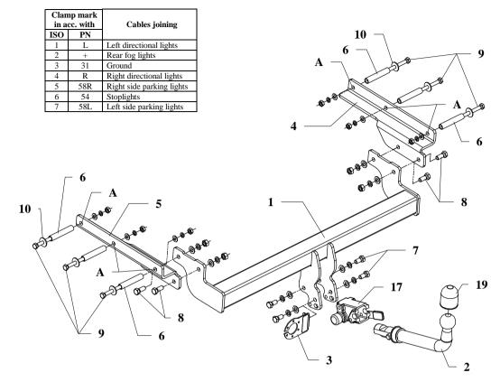
This towbar is designed to assembly in following car: **FORD MONDEO ESTATE**, produced since 1993 till 07.1996, catalogue no. **C20A** and is prepared to tow trailers max total weight **1800 kg** and max vertical load **75 kg**.
