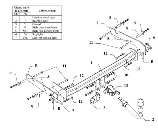
This towing hitch is designed to assembly in following cars: **FORD FIESTA COURIER delivery van**, produced since 08.1996 till 12.2002, catalogue no. **C24A** and is prepared to tow trailers max total weight **900 kg** and max vertical load **50 kg**.
