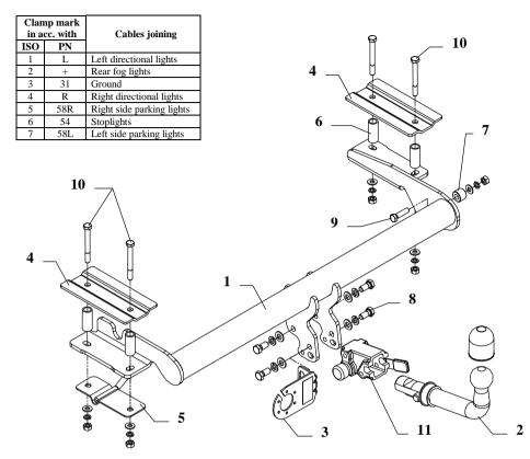
This towbar is designed to assembly in following cars: **FORD ORION**, produced since 11.1990 till 07.1993 and **FORD ESCORT**, 4 doors, produced since 08.1993 till 1995, catalogue no. **C40A** and is prepared to tow trailers max total weight 1200 kg and max vertical load 50 kg.
