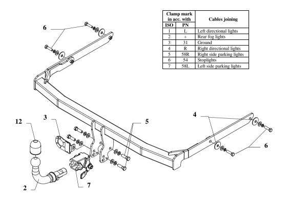
This towbar is designed to assembly in following car: **FORD FUSION** produced since 2002, catalogue no. **C43A** and is prepared to tow trailers max total weight **900kg** and max vertical load **50kg**.
