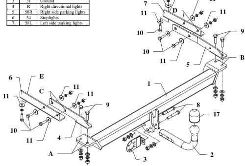
This towbar is designed to assembly in following cars: MERCEDES C208, W202, S202, C Class, CLK, 4 door, ESTATE, produced since 11.1993 till 05.2002, catalogue no. D14 and is prepared to tow trailers max total weight 1800 kg and max vertical mass 75 kg.
