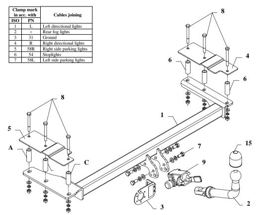
This towbar is designed to assembly in following cars: **OPEL ASTRA "A", 4 doors**, produced since 1991 till 2002, catalogue no. **E08A** and is prepared to tow trailers max total weight **1500 kg** and max vertical load **75 kg**.
