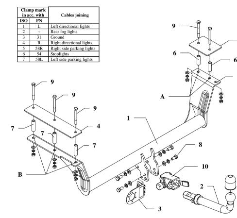
This towbar is designed to assembly in following cars: **OPEL OMEGA "B" ESTATE**, produced since 1994 till 2003, catalogue no. **E17A** and is prepared to tow trailers max total weight **2000kg** and max vertical load **75kg**.
