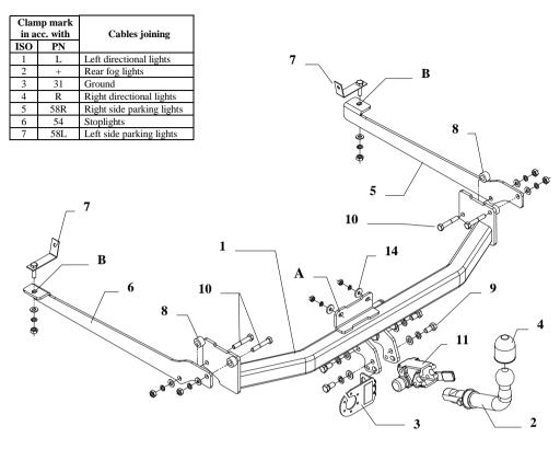
This towbar is designed to assembly in following car: **PEUGEOT 306 4 doors,** produced since 1994 till 2000, catalogue number **F09A** and is prepared to tow trailers max total weight **1400 kg** and max
