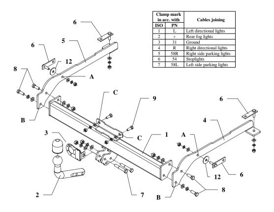
This towbar is designed to assembly in following cars: **PEUGEOT 605** produced since 1990 till 2000, catalogue number **F10** and is prepared to tow trailers max total weight **1500 kg** and max vertical mass **75 kg**.
