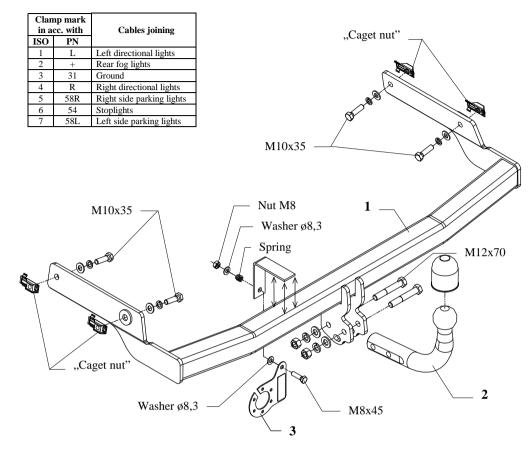
This towbar is designed to assembly in following car: **PEUGEOT 206, 3/5 doors, CC,** produced since 1998 till 03.2003 and since 03.2003 till 2009 and **PEUGEOT 206+** produced since 2009, catalogue number **F27** and is prepared to tow trailers max total weight **1100 kg** and max vertical load **50 kg**.
