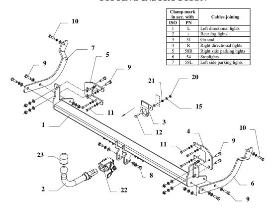
This towbar is designed to assembly in following car: **PEUGEOT 407SW (ESTATE),** produced since 2004 till 08.2008, catalogue number **F28A** and is prepared to tow trailers max total weight **1600 kg** and max vertical load **65 kg**.
