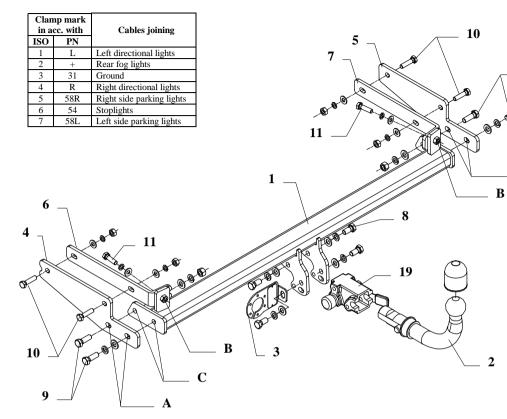
This towbar is designed to assembly in following cars: **RENAULT THALIA, 4 doors,** produced since 2001, catalogue no. **G37A** and is prepared to tow trailers max total weight **1150 kg** and max vertical load **75 kg**.
