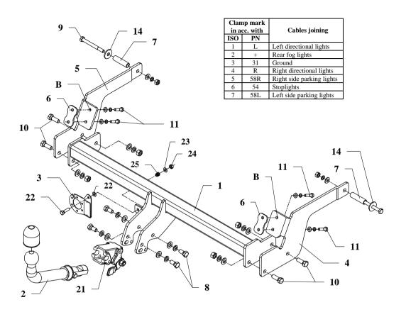
This towbar is designed to assembly in following cars: **RENAULT LAGUNA ESTATE**, produced since 2001 till 2007, catalogue number **G38A** and is prepared to tow trailers max total weight **1500 kg** and max vertical load **75 kg**.
