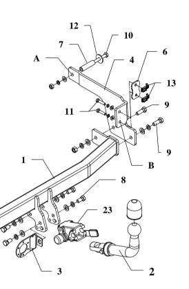
This towbar is designed to assembly in following cars: **RENAULT LAGUNA 5 doors,** produced since 2001 till 2007, catalogue no.**G39A** and is prepared to tow trailers max total weight **1500 kg** and max vertical load **75 kg**.
