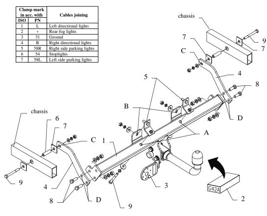
This towbar is designed to assembly in following car: **RENAULT KANGOO 4WD**, produced since 2003, catalogue no. **G42A** and is prepared to tow trailers max total weight **1350 kg** and max vertical load **75 kg**.
