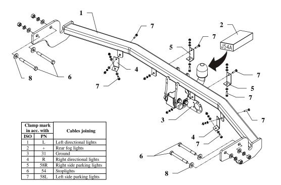
This towing hitch is designed to assembly in following cars: **HYUNDAI SANTA FE**, produced since 03.2006 till 08.2012, catalogue no. **J54A** and is prepared to tow trailers max total weight **2700 kg** and max vertical load **100 kg**.
