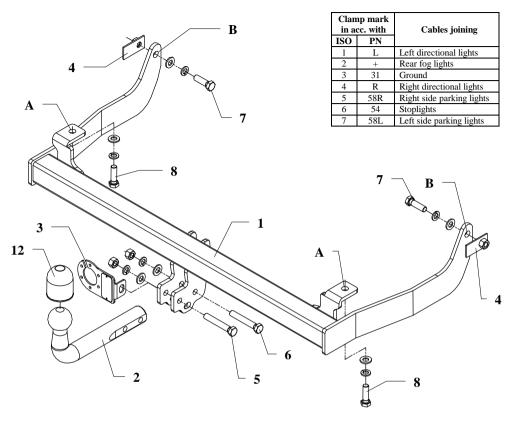
This towing hitch is designed to assembly in following cars: **VOLKSWAGEN CADDY II, SEAT INCA** both produced since 11.1995 till 12.2003, catalogue no. **K31** and is prepared to tow trailers max total weight **1100kg** and max vertical load **50 kg**.
