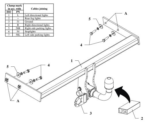
This towing hitch is designed to assembly in following cars: **VOLVO S80 (4 doors)** produced since 08.2006 and **V70 (estate)**, produced since 08.2007, catalogue no. **L20A** and is prepared to tow trailers max total weight **2100 kg** and max vertical cup load **90 kg**.
