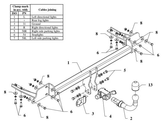
This towbar is designed to assembly in following car: MAZDA 323 produced since 09.1998 till 12.2001, catalogue no. M46A and is prepared to tow trailers max total weight 1600 kg and max vertical load 75 kg.
