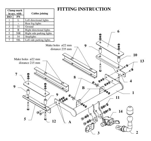
This towbar is designed to assembly in following car: CITROEN SAXO 3-5 doors, produced since 1996 till 2004, catalogue no. P09A and is prepared to tow trailers max total weight 1100 kg and max vertical load 50 kg.
