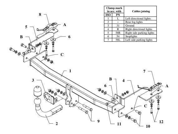
This towbar is designed to assembly in following cars: **FIAT PUNTO II, 3/5 door,** produced since 09.1999 till 09.2005, catalogue no. **R25** and is prepared to tow trailers max total weight **1600 kg** and max vertical load **60 kg**.
