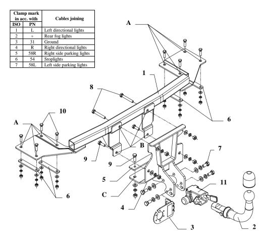
This towbar is designed to assembly in following cars: **FIAT ALBEA, 4 doors,** produced since 2002, catalogue no. **R32A** and is prepared to tow trailers max total weight **1300 kg** and max vertical mass **50 kg**.
