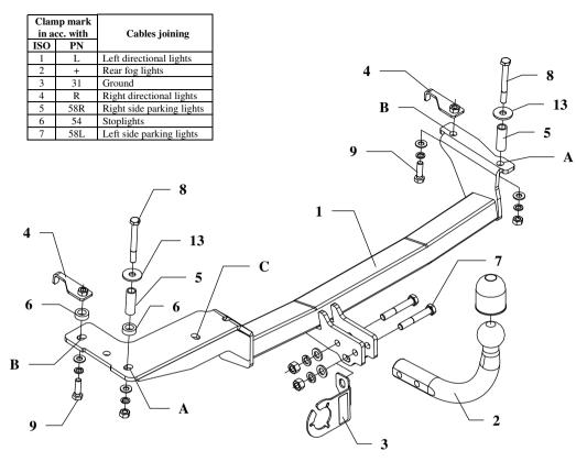
This towing hitch is designed to assembly in following cars: **SEAT IBIZA 3/5 doors**, produced since 04.1993 till 01.1996, catalogue number **SC01** and is prepared to tow trailers max total weight **1100 kg** and max vertical load **75 kg**.
