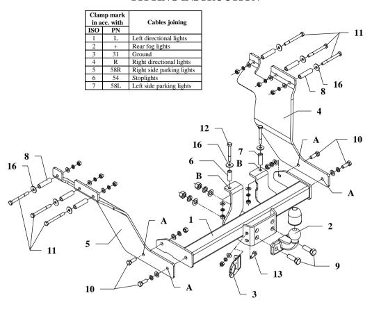
This towing hitch is designed to assembly in following cars: **KIA PREGIO**, produced since 1997, catalogue no. **T12** and is prepared to tow trailers max total weight **1500 kg** and max vertical mass **70 kg**.
