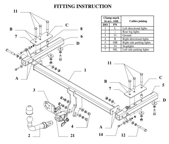
This towbar is designed to assembly in following car: **KIA CARENS** produced since 09.2001 till 10.2006, catalogue no. **T43** and is prepared to tow trailers max total weight **1250** kg and max vertical load **75** kg.
