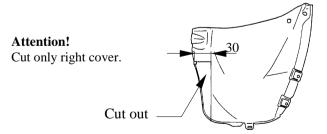
Fig. 3. Right side cover – cut out.
