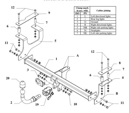
This towbar is designed to assembly in following cars: **SUZUKI WAGON R+** and **OPEL AGILA** produced since 04.2000 till 08.2002, catalogue no. **W14A** and is prepared to tow trailers max total weight **1000 kg** and max vertical load **30 kg**.
