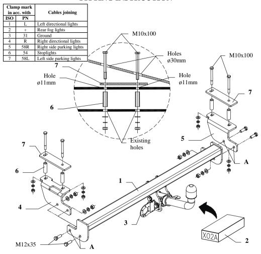
This towbar is designed to assembly in following cars: **DAEWOO NEXIA, 3-5 door,** produced since 1995 till 1997, catalogue no. **X02A** and is prepared to tow trailers max total weight **1200 kg** and max vertical load **70 kg**.
