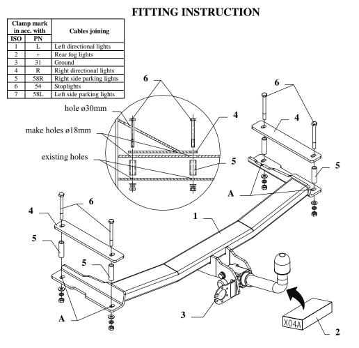
This towbar is designed to assembly in following cars: **DAEWOO ESPERO, 4 door,** produced since 1995 till 1997, catalogue no. **X04A** i and is prepared to tow trailers max total weight **1200 kg** and max vertical load **70 kg**.
