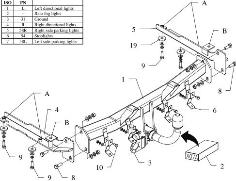
This towbar is designed to assembly in following cars: DAEWOO NUBIRA ESTATE, produced since 1997 till 01.1998, catalogue no. X07A and is prepared to tow trailers max total weight 1200 kg and max vertical mass 70 kg.
