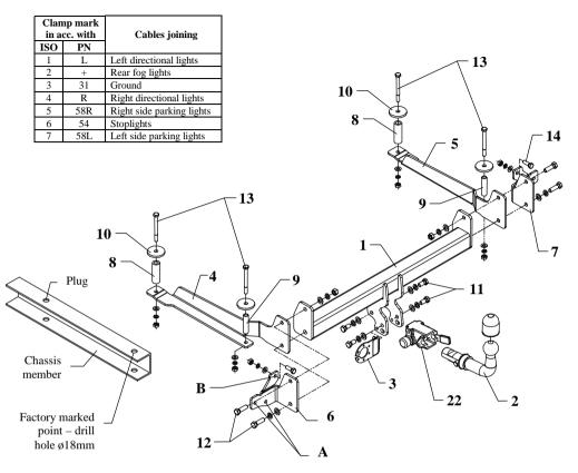
This towbar is designed to assembly in following cars: HONDA ACCORD 4-5 doors, produced since 11.1998 till 12.2002, catalogue no. Y08A and is prepared to tow trailers max total weight 1500 kg and max vertical load 60 kg.
