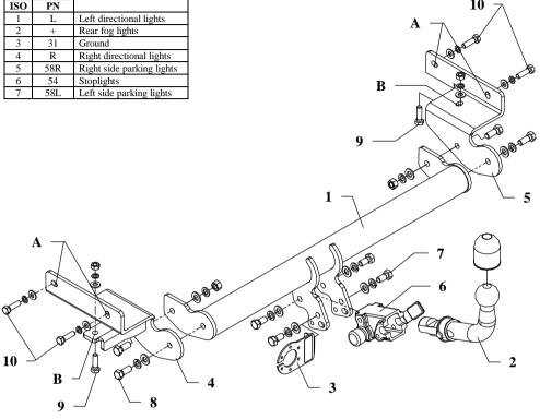
This towing hitch is designed to assembly in following cars: MITSUBISHI LANCER, 4/5 door (CK), produced since 01.1996 till 2003, catalogue no. **Z21A** and is prepared to tow trailers max total weight 1300 kg and max vertical load 50 kg.
