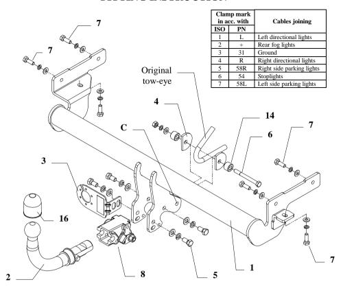
This towbar is designed to assembly in following car: **MITSUBISHI CARISMA 4/5 door,** produced since 08.1995 till 1999 and since 2000 till 2005, catalogue number **Z23A** and is prepared to tow trailers max total weight **1450 kg** and max vertical load **75 kg**.
