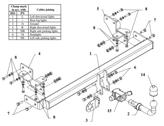
This towbar is designed to assembly in following cars: **MITSUBISHI SPACE WAGON** produced since 05.1992 till 09.1998 and **HYUNDAI SANTAMO** produced since 1999, catalogue no. **Z24A** and is prepared to tow trailers max total weight **1800** kg and max vertical load **90** kg.
