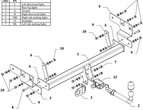
This towbar is designed to assembly in following cars: MITSUBISHI PININ 5 doors, produced since 2000, catalogue no. Z26A and is prepared to tow trailers max total weight 1500kg and max vertical load 75 kg.
